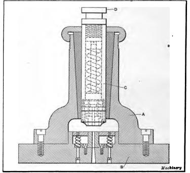
Fig. 14. Sub-press for Aligning and Guiding Upper and Lower Members of Compound Dies
